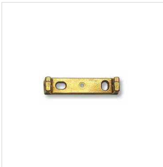
31-021-10 Staffa per / Stirrup for 31-021-01 L60 x W10 x H15 filetto/thread M4
